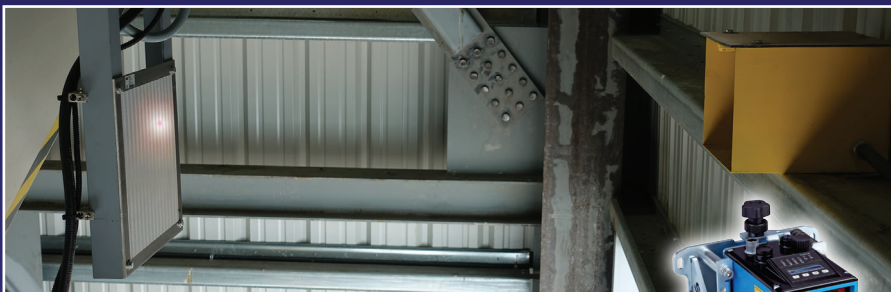
Absolute scale position is accurately determined by an industrial grade laser range measuring device.
